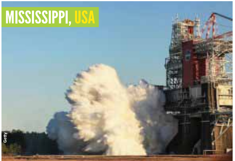
NASA tested its Space Launch System rocket, a core part of the Artemis I mission that will take humans back to the moon for the first time since the 1970s. The eight-minute test of the 'megarocket' ended when the engines shut down after just a minute. Teams are studying what caused the early shutdown.
